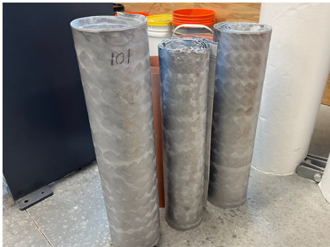
Lead Sheets After Hammering
