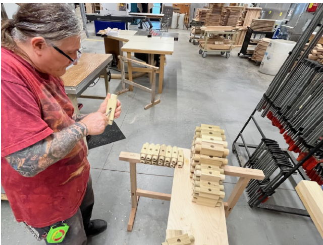
Markus Making the Feet for the Wooden Pipes
